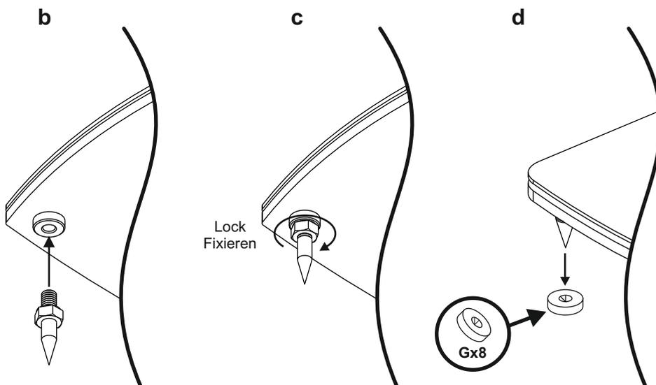
NOTE: In case you have a sensitive floor surface (like hardwood or tiles) which could be damaged by the spikes, please use the spike plates included in the kit (G)
